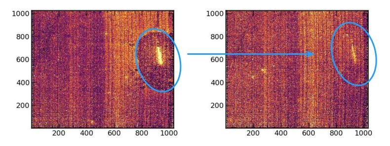
cosmic rays can persist over multiple exposures (here, ghosting two exposures after the initial event) — missed by pipeline!!
