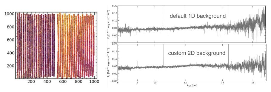
pipeline uses collapsed 1D background, losing key spatial background information
